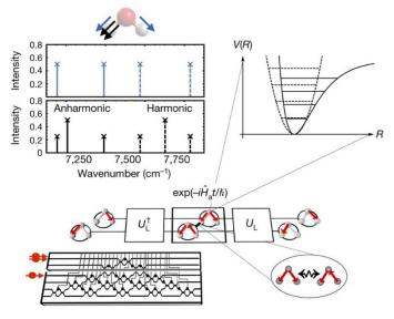
Figure 5: Quantum photonic integrated circuit with thermo-optic phase shifters (bottom) allows for simulating the vibrational quantum dynamics of molecules (taken from Nature (2018): <u>https://doi.org/10.1038/s41586-018-0152-9</u>)
