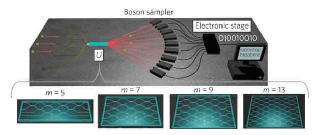
Figure 3: Boson Sampling experiment with integrated photonic circuits of different mode numbers (taken from Nature Photonics (2014): <u>https://doi.org/10.1038/nphoton.2014.135</u>)
