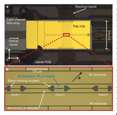
Fig. 4: Optical micrograph of an assembled ion trap device with an eightchannel fibre array attached. b, Higher-magnification view near the trap zones (taken from Nature (2020) <u>https://doi.org/10.1038/s41586-020-</u> 2823-6)
