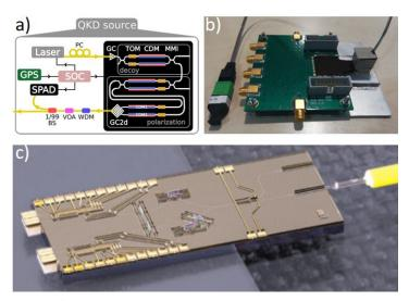
Figure 2: a) shows the scheme of the QKD state generator system and b) the integrated chip including connectors (taken from Quantum Physics (2019): <u>https://doi.org/10.48550/arXiv.1907.10039</u>) . c) Photonic circuit with hybrid integration of transceivers for CV- and DV-QKD, including InP based single photon detectors (courtesy of HHI)
